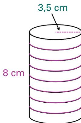
$$\begin{aligned} V_{\text{cylindre}} &= A_{\text{base}} \times H \\ &= A_{\text{disque}} \times H \\ &= \pi \times r^2 \times H \\ &= 3,14 \times 3,5 \times 3,5 \times 8 \\ &= 307,72 \\ &= 307,72 \text{ cm}^3 \end{aligned}$$
